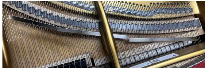
Fig. 3: Place bar magnets in a row close to the bridge (but leave a slight gap), covering notes from E5 to B7.
